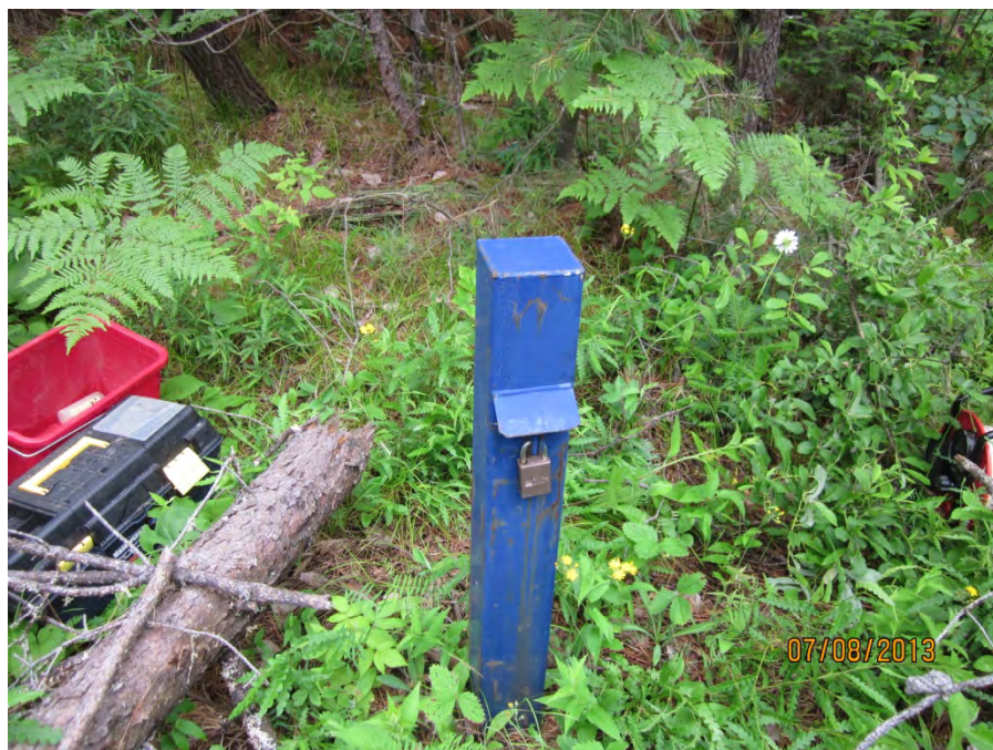
Photo 2 Groundwater monitoring wells BH2-I, July 2013
